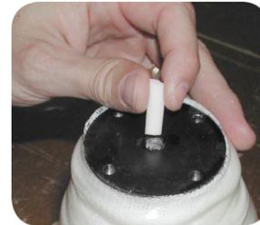
Apply the 4-Hole Adapter to the socket.
