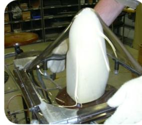
Lightly sand the socket. Wrap with casting tape.
