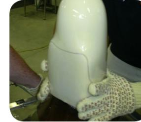
Tape off the entire surface of the 4-Hole Adapter to protect from resin.
