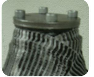
Apply the layup. Tie off in the space between the forming plate and 4-hole Adapter. Pull the rest of the layup down. Laminate.
