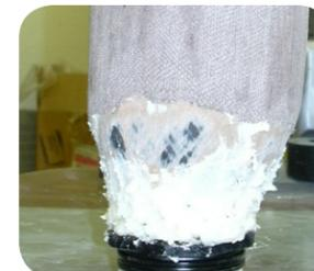
Apply the carbon tape around the 4-Hole Adapter.
