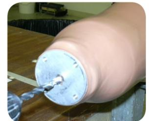
Push the filter into the hole. Cut it flush with the socket.
